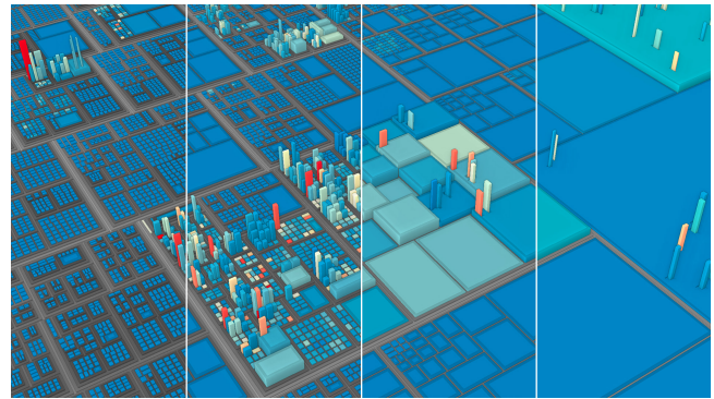
Figure 5: Stepwise generalization of a software map by use of aggregation, ranging from no aggregation (left) to strong aggregation (right). Outlier nodes – also called landmarks – are preserved [37].
