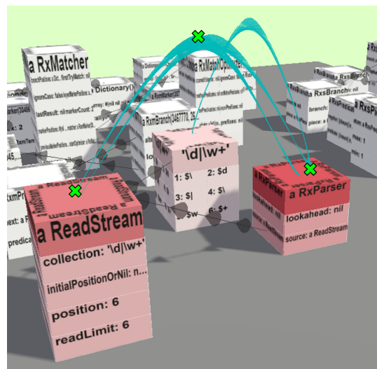
Figure 3: Visual mapping of object behavior to block colors and the trail in the object map. The intensity of the red color indicates the recency of the last message received by the corresponding object. The gradient trail curve connects the most recent object activations (control points of the curve are marked with a cross ( \times )).
